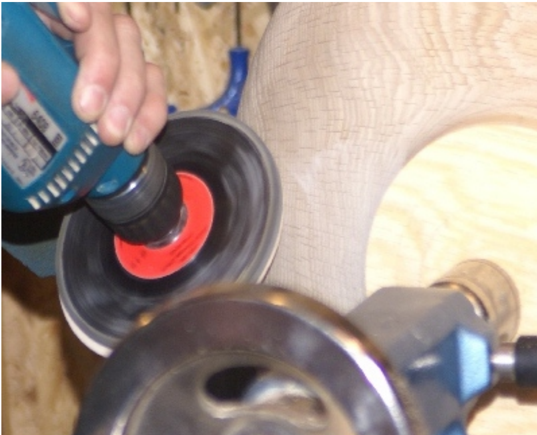
Sanding the outside of the bowl. Harmon turns to final shape so sanding at this point is part of the finish process. Did not record the grit for the final sanding.
