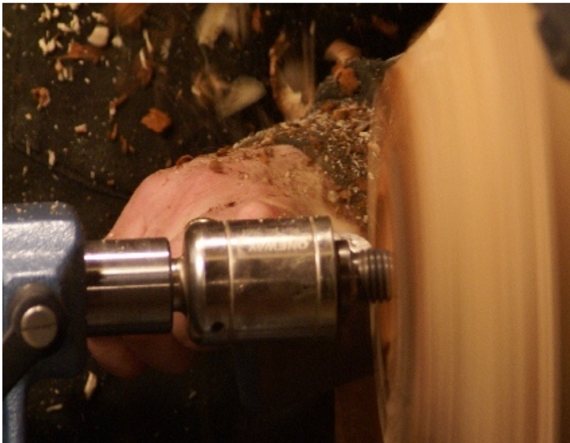
A close up of the spinning bowl and the gouge engaging the wood.
