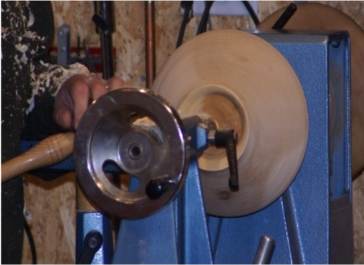
Here the bottom of the bowl is taking shape. Harmon turns a foot to grasp with his chuck.
